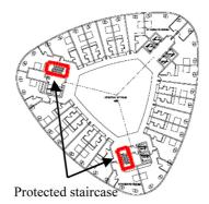
Figure 19. Arrangement of two protected staircases on typical hotel floors.
