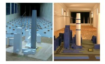
Figure 31. HFBB wind tunnel test.
