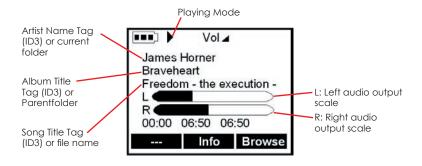
The Jukebox Recorder 2 will display the following image when connected to your ٠ computer's USB port.
