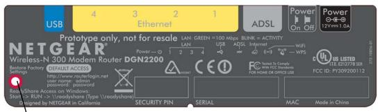
**Factory Default Reset.** Press for 6 seconds to reset the router to its factory default settings.
